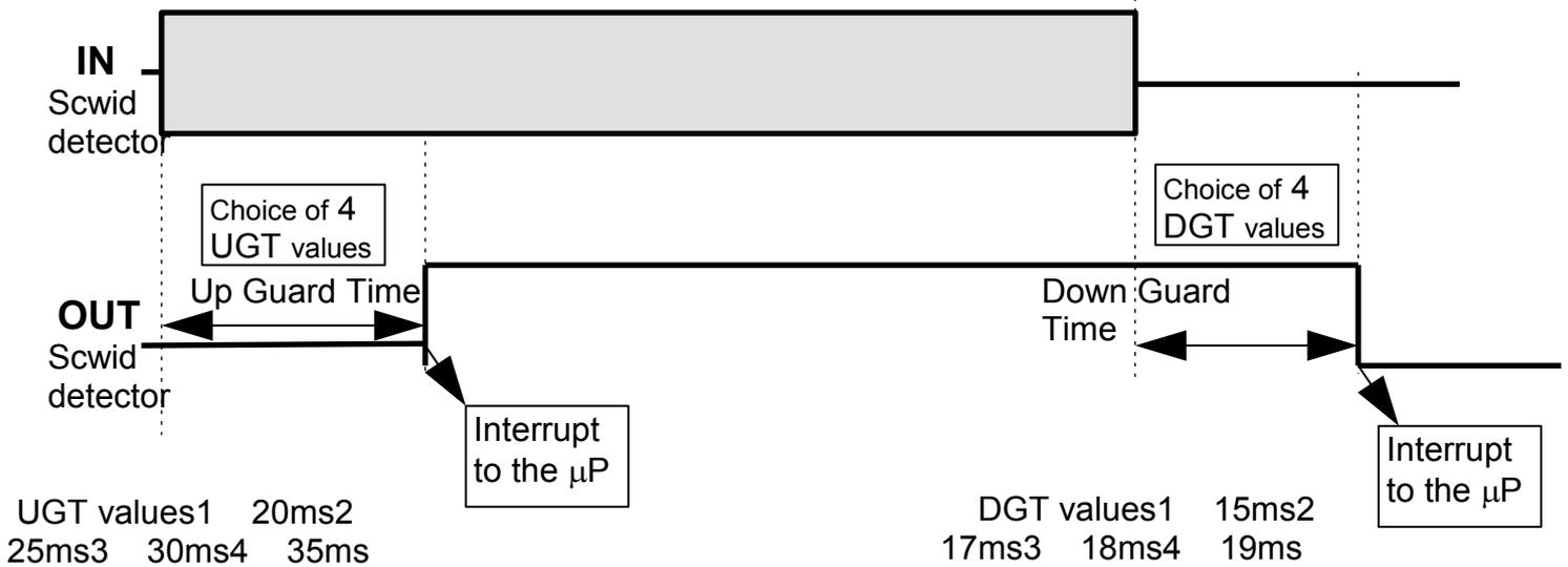
If any drop, in the CAS signal, occurs before the end of the UGT specified value then the time counter restarts and the **OUT scwid detector remains low**.
