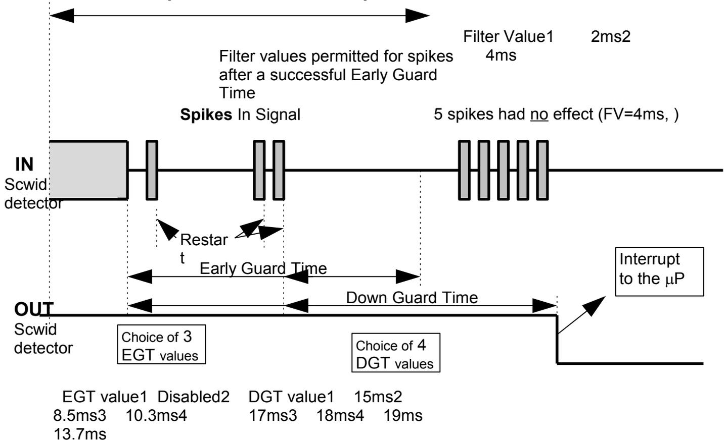
**Note :** In the case above the EGT counter restarted 3 times. After a successful 13.7ms EGT, 5 spikes occurred but without any effect because the duration is less than the maximum permitted.
