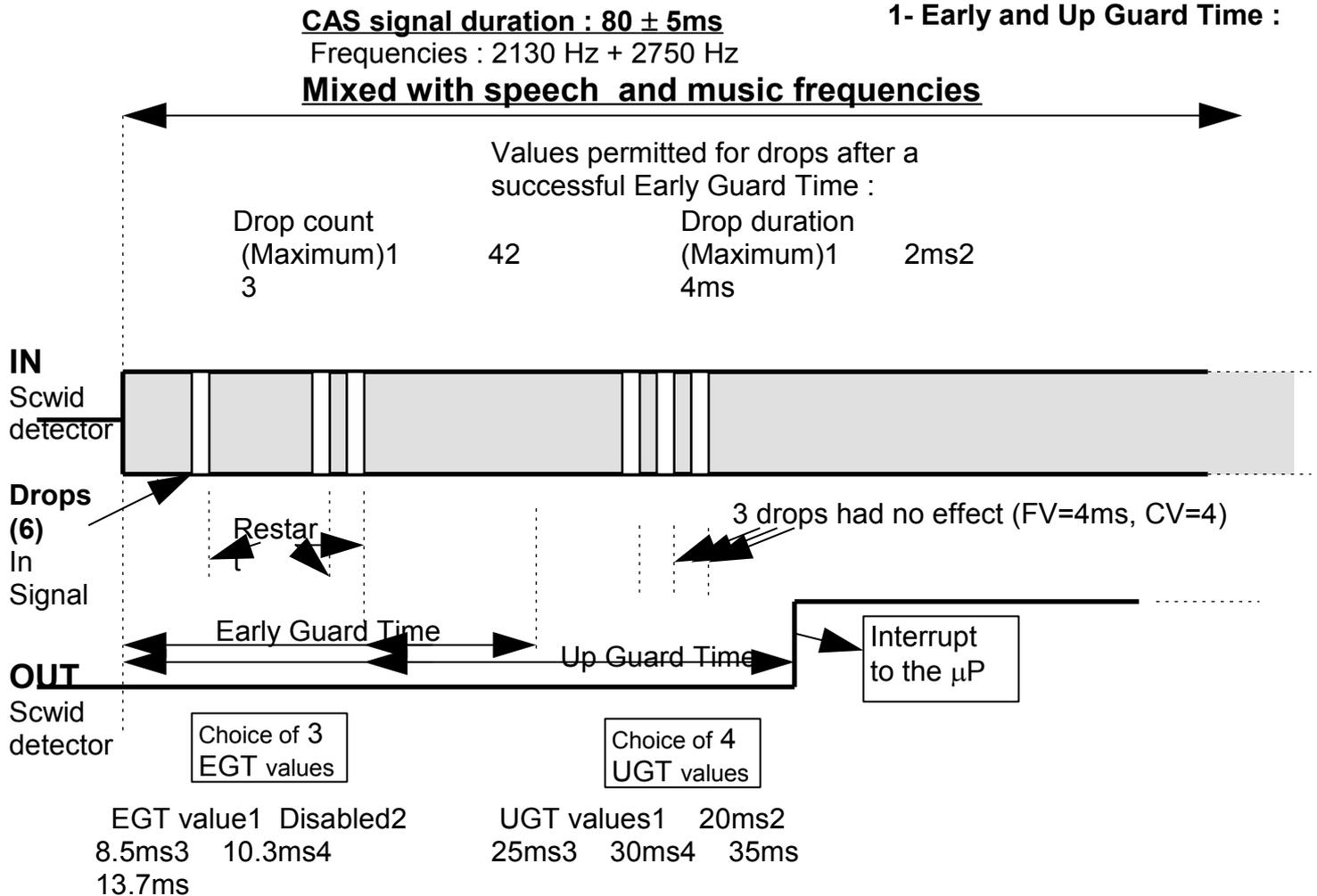
**Note :** In the case above the EGT counter restarted 3 times. After a successful 10.3ms EGT, 3 drops occurred but without any effect because the duration and the number is less than the maximum permitted.
